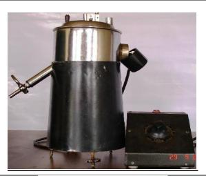
5 **Separating and throttling calorimeter**Steam Capacity - 6 Kg/hr from feedwater at 30° C
